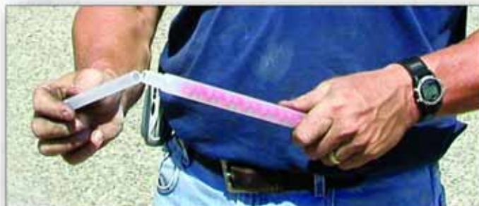
The "HP" Nozzle breaks off to accommodate varying hole diameters and depths.
